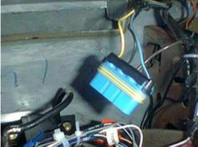
8-attach new wire to each side of cut w/connectors
